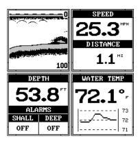
Press the left or right arrow key until the desired window group that you want to reset appears. When it appears, simply press the down arrow key and the unit will reset only that group. Press the EXIT key to erase the menu.
